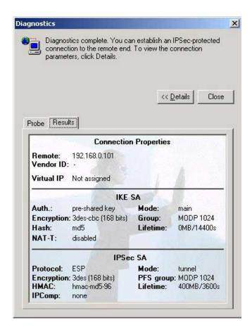
We can now use the SSH Sentinel icon in the task bar, select the VPN server and establish the VPN tunnel.
